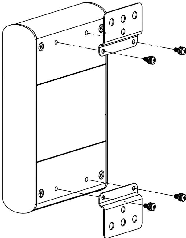
Once both mounting brackets are secured onto the extender, it is ready for mounting onto a surface.
