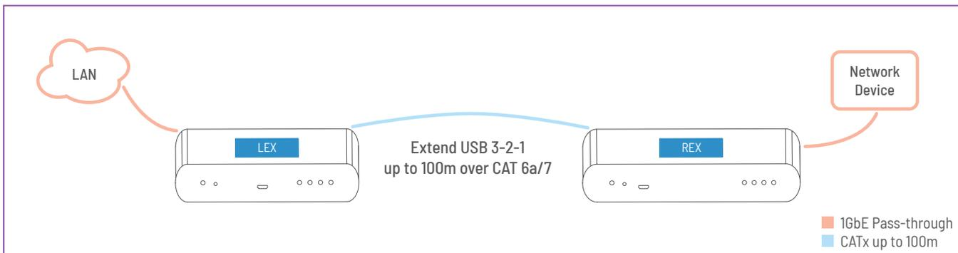
Connect any network device or access port into the RJ45 port labeled "1Gb Ethernet" using up to 100 meters of standard CAT 6a/7 cabling.
