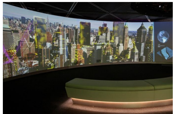
“Enter the City of the Future,” shown on a nine-meters curved screen by three DLP projectors with short-throw zoom lenses
